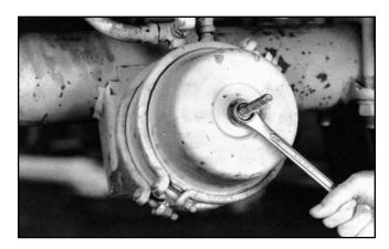
2. If the vehicle is equipped with spring brake chambers, manually cage the spring brakes following the manufacturer's recommended procedures.
