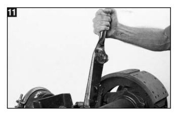
**11.** Once the 1 1/4" collar nut has been properly tightened to the clevis, tighten the 15/16" jam nut against the collar lock nut using 40 to 50 ft lbs of torque.
