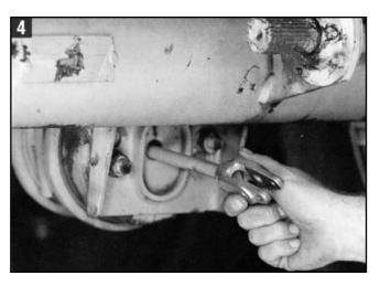
**4.** When installing a CSI Midland/Gunite automatic brake adjuster with a threaded clevis, install the new clevis on the push rod in the same locations as the clevis which was removed. Do not tighten the jam nut at this time.
