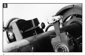
5. Install the brake adjuster onto the camshaft with the adjusting hex pointing away from the brake chamber.
