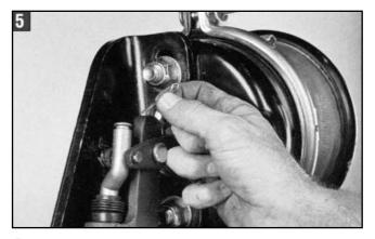
5. Insert the cotter pins into the large and small holes and secure the cotter pins.
