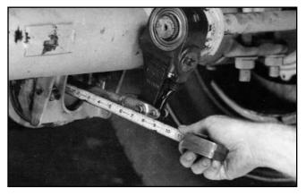
**9.** Using a ruler, measure the distance from the face of the air chamber to the center of the large pin in the clevis (A). (See Figure 15.)
