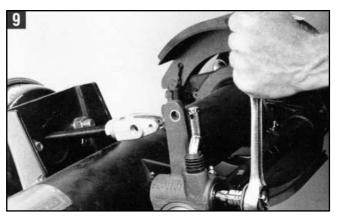
9. Apply anti-seize compound to the camshaft and clevis pins. Install the brake adjuster onto the camshaft with the adjusting hex pointing away from the brake chamber.
