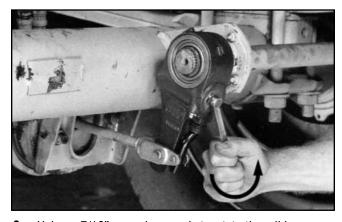
**3.** Using a 7/16" wrench or socket, rotate the adj hex counterclockwise. You should have at least 15 ft. lbs. resistance and a ratcheting sound will be heard as the adj hex is rotated.
