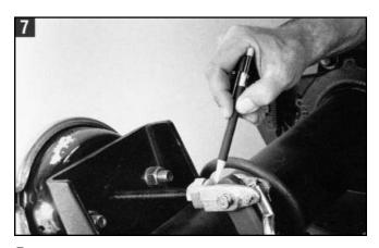
7. Before attaching the 1 1/4" collar nut to the clevis, check to make sure the threaded push rod is fully engaged in the 3/4" hex nut. If the push rod does not have full engagement, a new push rod must be installed and cut to length. Refer to the section on cutting a new push rod to length in this manual.
