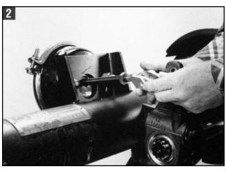
2. Remove the existing clevis and brake adjuster. Keep the existing mounting hardware. Do not remove the clevis jam nut.
