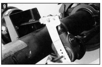
**9.** Align the brake adjuster by adjusting the 3/4" hex nut on the push rod until the appropriate centering hole on the template aligns with the center hole on the camshaft. The template is provided with centering holes for 5, 5.5, 6 and 6.5 inch brake adjusters.
