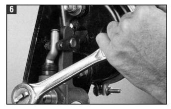
**6.** Pre-adjust the brakes by rotating the adjust hex clockwise until the brake lining contacts the brake drum. Back the brake adjuster off by rotating the hex counterclockwise 1/2 turn. Backing off a new brake adjuster may require up to 50 ft lbs of torque. A ratcheting sound will be heard when backing the brake adjuster off.
