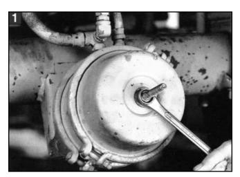
1. If the axle is equipped with spring brake chambers, manually cage the spring brakes following the manufacturer's recommended procedures. Note: When caging the spring brakes, always be sure to block the vehicle wheels to prevent unwanted movement.
