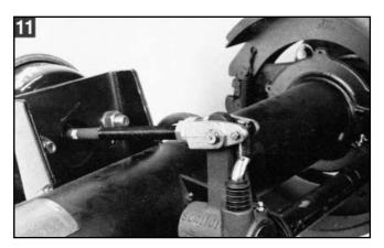
**11.** Fully apply the brakes and allow the chamber push rod to travel its maximum stroke. Clearance must exist between the brake adjuster and all adjacent chassis components. Release the brakes.
