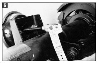
**6.** Align the clevis on the threaded push rod until the appropriate centering hole on the template aligns with the center hole on the camshaft. The template is provided with centering holes for 5, 5.5, 6 and 6.5 inch brake adjusters.
