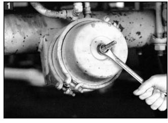
1. Block the vehicle's wheels. If the axle is equipped with spring brakes, manually cage the brakes following the manufacturer's recommended procedures.
